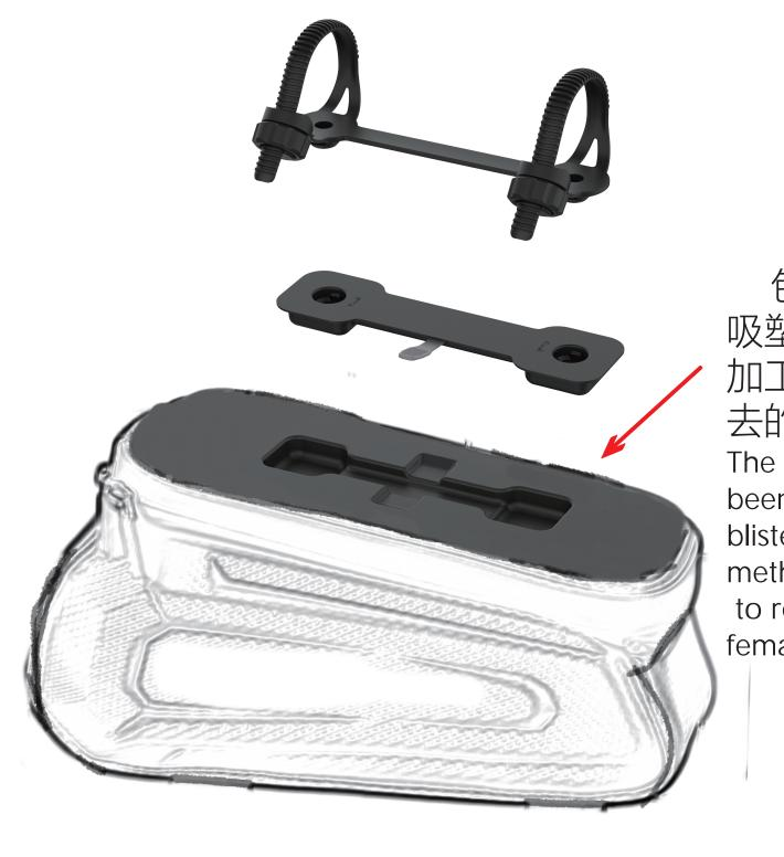
包上预先通过 吸塑或其他方式 加工好母扣凹进 去的形状。 The shape that has been created by blister or other methods is reserved to recess the female buckle
